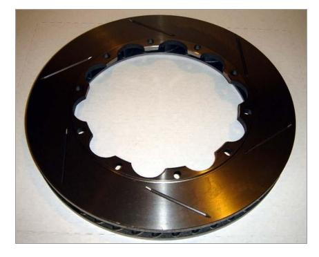
**1)** Lay new rotor face down with mounting flanges facing up.
