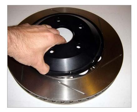
3) Install new drive pins into hat. They should slide in, but <u>light</u> tapping with a hammer is not uncommon. Be sure the drive pins are fully seated on the hat as each bolt is tightened. If the drive pins are not clocked properly against the hats, permanent damage to the hats may result.
