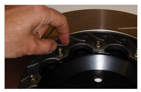
**5)** After installing all bolts **finger tight**, flip the rotor assembly over, hat-side up. Before using the thread locker, shake well, then snip off the end of the plastic nozzle. Place ONE DROP of 290 Loctite in the threads of each drive pin. components. Then proceed to the next step to torque all fasteners.
