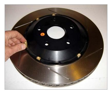
**4)** Flip rotor over and install bolts and washers' finger tight. The concave surface faces downward, making the washers appear as small domes.
