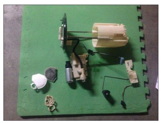
The regulator can be seen on the side of the fuel pump housing assembly. Install the new pump and sock and reconnect the OEM supply line. Reinstall the sending unit.
